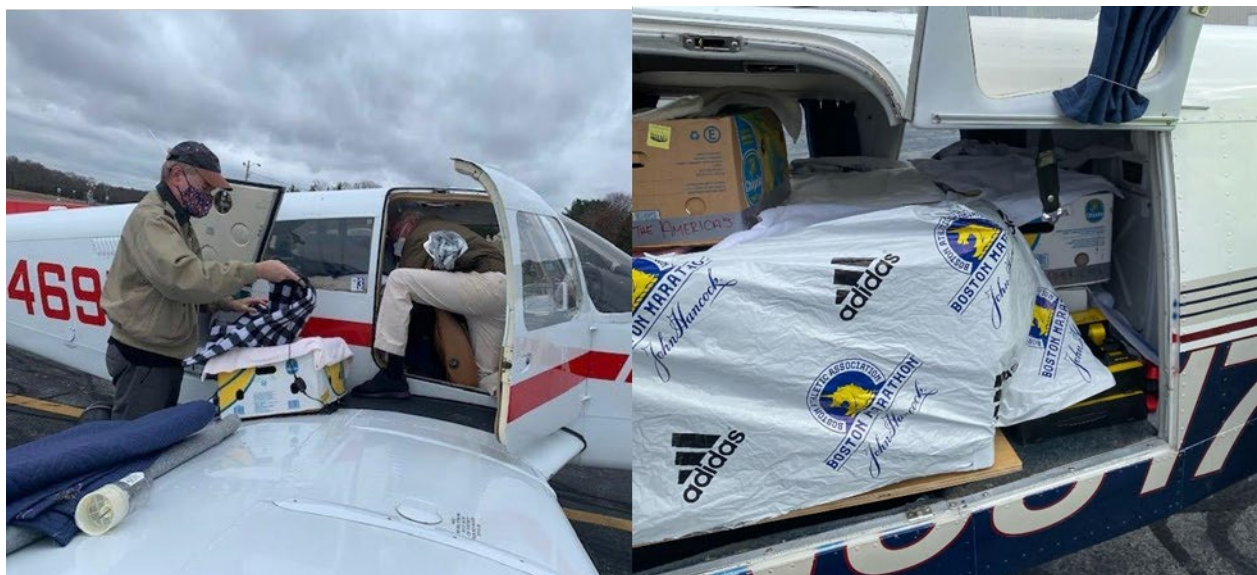
Figure 2.2.1.1.1 Containers covered with light towels or marathon blankets to maintain heat. In addition, insulating material can be added between the fuselage and the sea turtle containers to maintain heat.
