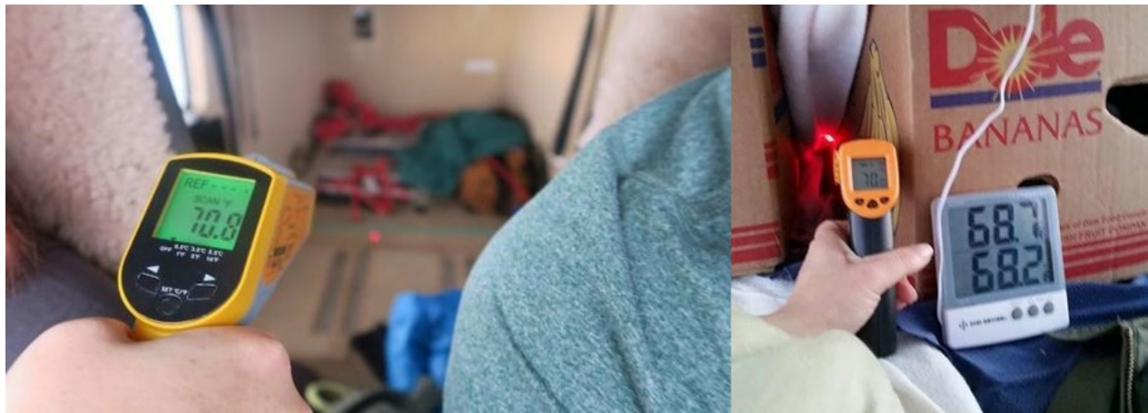
Figure 3.2.1.1 Using a heat gun and a thermometer to check cabin temperature. Photos courtesy of Turtles Fly Too.
