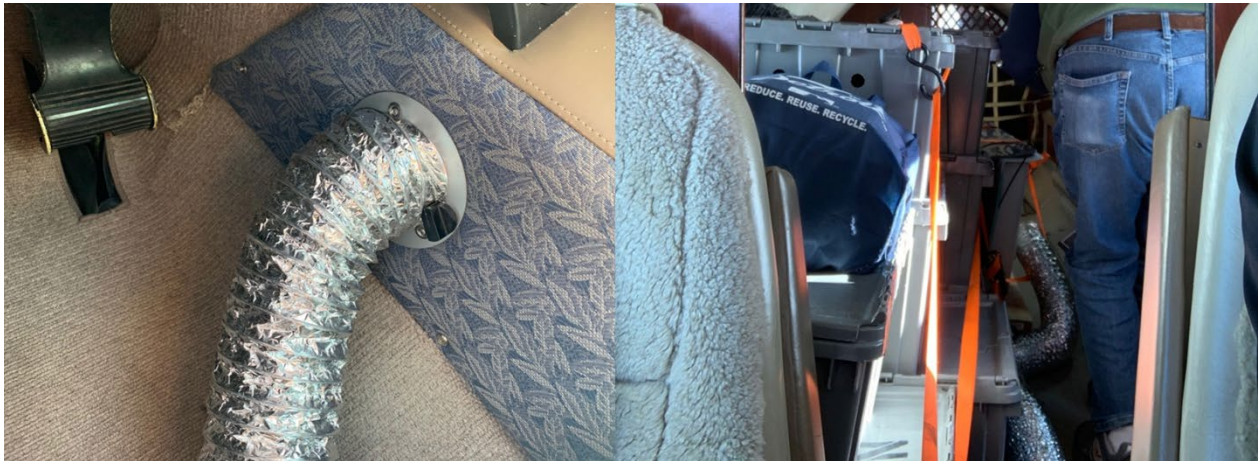
Figure 2.3.1 Dryer hose on vent and running through the fuselage to the back of the plane to transfer heat.
