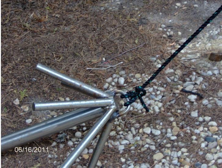
New eye welded on grappling anchor to make handling easier and safer
